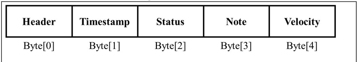
In Header, bit-7 is a start bit, forced to 1, and bit-6 is reserved, forced to 0. In Timestamp, bit-7 is a start bit, forced to 1. In other words, the bit 0 to bit 5 of Header refer to the six high bits of 13-bit timestamp. The bit 0 to bit 6 of Timestamp means the seven low bits of 13-bit timestamp.
